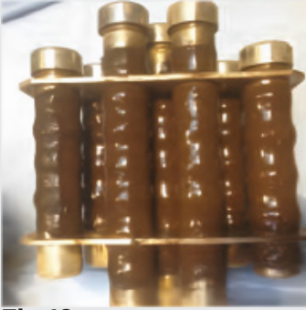
Fig 19. Dirty Magnet Grate.
