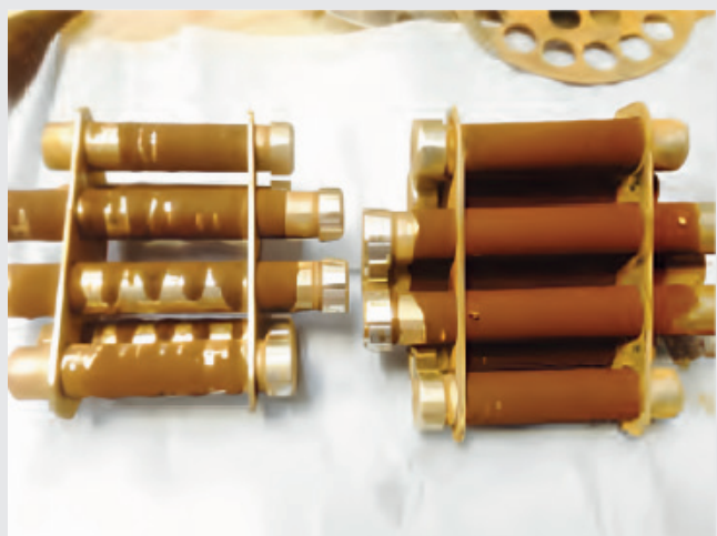
Fig 18. Both Magnet Grates removed for cleaning (Day 34).
