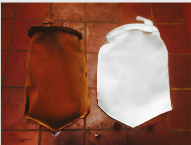
Fig 17. First filter removed after 5 days (Day 34) with new filter ready to be added.
