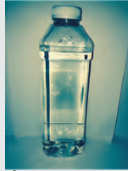
Fig 22. Sampled water from the heating is also clear with a very slight haze.
